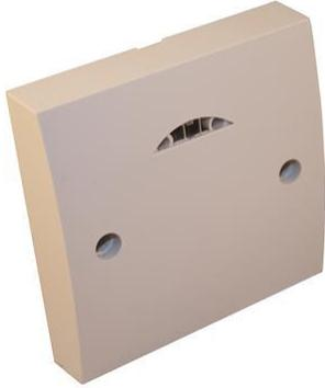
The MWS-1A-PRM microwave presence detectors are designed to provide automatic control of lighting, heating or ventilation loads. Detecting movement using a highly sensitive microwave detector. It works by emitting low power microwave signals and measuring the reflections as the signals bounce off moving objects. Wall mounting applications to give detection over long distances. When movement is detected the load is turned on. The unit is controlled and programmed using handheld IR Handsets
