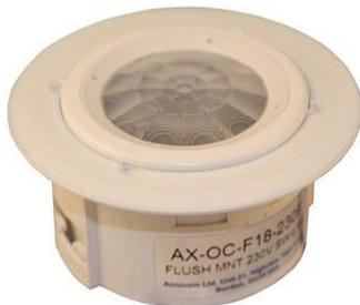
The AX-OC-F18 range of occupancy sensors are passive infra-red sensors for monitoring occupation through body heat. Detection of occupation will activate the internal relay. There are switched live and volt free output variants. The units include a light level control which can be turned off if required. There are 230Vac and 24Vac/dc variants.
